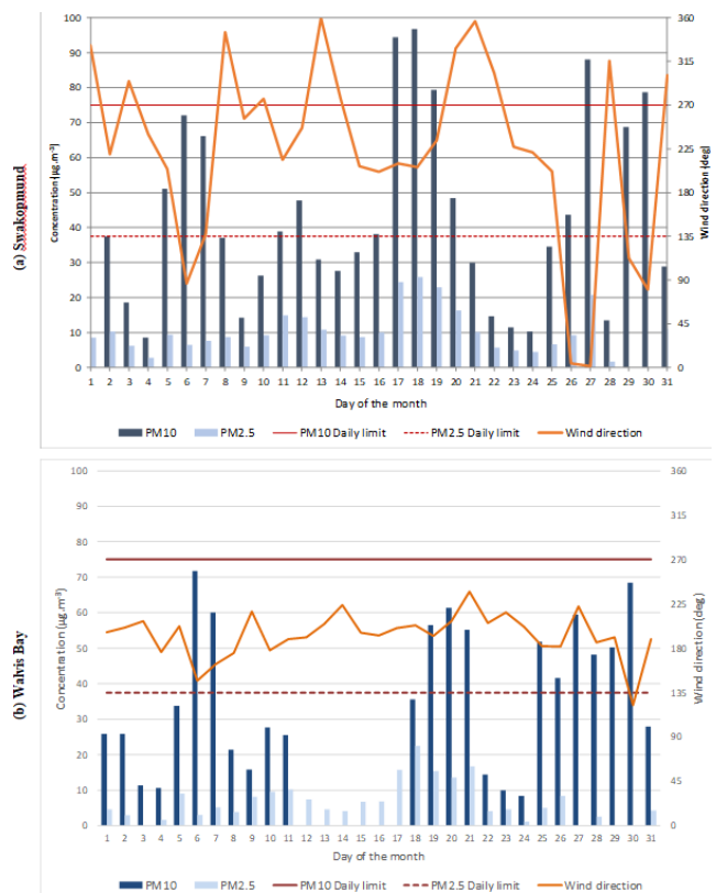
Figure 3: Daily PM 10 and PM 2.5 concentrations at (a) Swakopmund and (b) Walvis Bay with average daily wind directions indicated for the month of July 2017.
