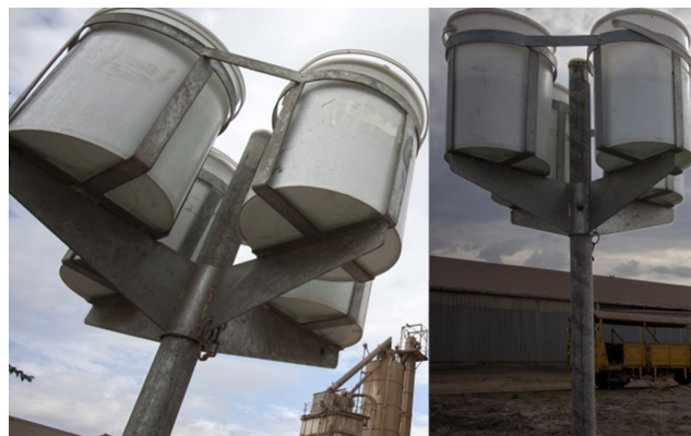
Figure 1: Converted Directional Dust Bucket Stands.
