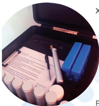
X-LAB EARTH SCIENCE has developed kits for customers that are routinely deploying 10 to 30 samples per month. The kit contains TD Tubes - prelabelled, spanners to mount the tubes, easy-to-follow instructions, log sheets and cool packs, all conveniently packaged in a rugged transport case.
