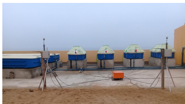
Figure 2: E-samplers (mounted on tripod stands) that were used to concurrently measure \text{PM}_{2.5} (left) and \text{PM}_{10} (right).
