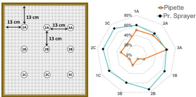
**Figure 2:** Spatial variation test to verify and optimize nanoparticle deposition uniformity. The spider-chart depicts the uniformity of the pressurized sprayer over the pipette deposition.
