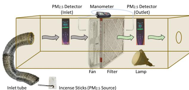
**Figure 1:** A wind tunnel with a fan to create the draft, and incense sticks to simulate the  $PM_{2.5}$  were used in this experimental set-up. Laser particle detectors at the inlet and outlet were used to measure the filtration efficiency and a manometer was used to measure the pressure drop.
