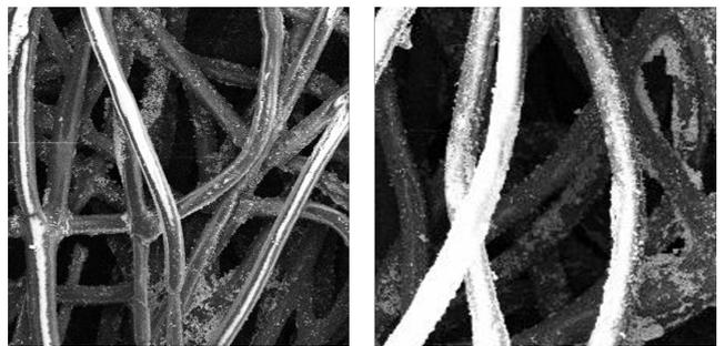
**Figure 3b:** Scanning Electron Microscope (SEM) images of the TiO<sub>2</sub> coated filter before (left) and after (right) exposure to PM<sub>2.5</sub> particles, show the adsorption of the PM<sub>2.5</sub> particles to the nanoparticle adhesion areas of the filtration media.
