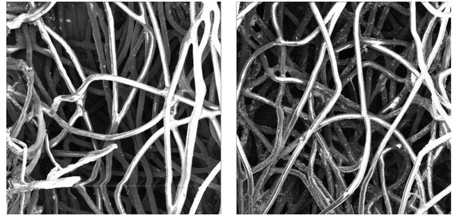
**Figure 3a:** Scanning Electron Microscope (SEM) images of the baseline filter (left) and the TiO<sub>2</sub> coated one (right) confirm the adhesion of the nanoparticles to the fibres of the filtration media.
