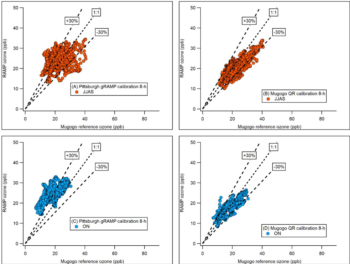
**Figure S2:** Comparison of RAMP calibration models for ozone with reference monitor data at the Mt Mugogo Climate Observatory. The “Pittsburgh gRAMP” model (A,C) is developed on collocations in Pittsburgh, PA, USA. The “Mugogo QR” model (B,D) is based on a collocation with the reference monitor at Mugogo; the data shown here includes both training (28 days) and testing (32 days) data. JJAS (A,B) is the dry season and ON (C,D) is the wet season.
