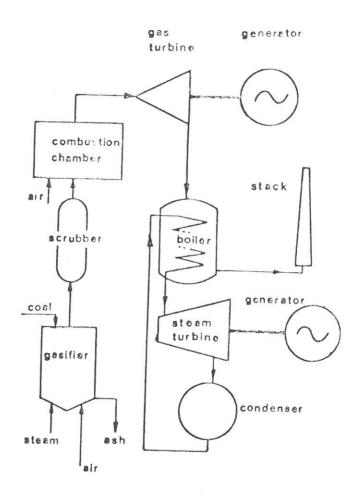
FIGURE I DUAL-CYCLE POWER PLANT
