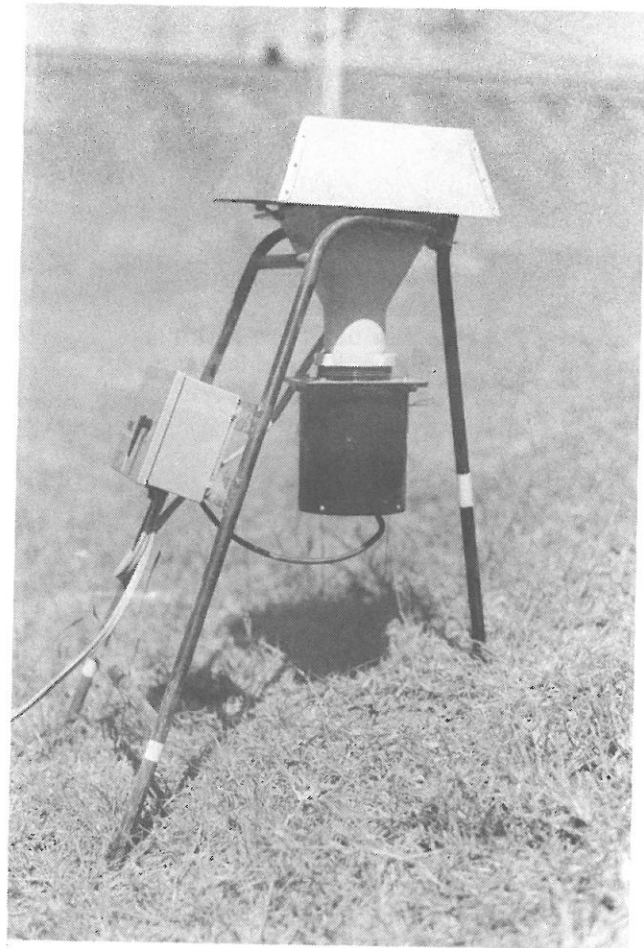
FIGURE 7: Tripod sampler with flow controller
