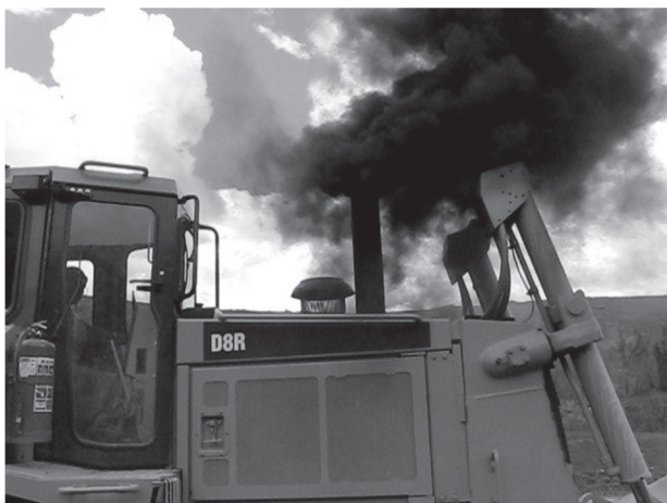
Figure 1: Optical presentation of Phase 2 of the fuel enhancement evaluation at Letšeng Diamond Mine before addition of product C.
