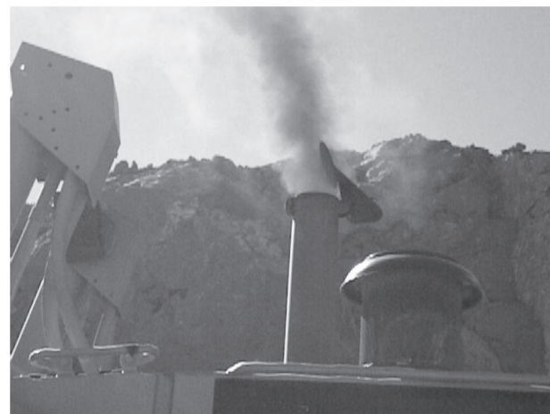
Figure 2: Optical presentation of the reduction in smoke 21 days after addition of product C during the fuel enhancement project at Letšeng Diamond Mine.
