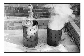
The principle is as follows: smoke is generated at the hot/cold boundary. In the normal bottom-up coal fire ignition process, the smoke rises through the cold coals and thus escapes. In the top-down ignition process, the smoke rises through the hot zone and is consequently burnt.
