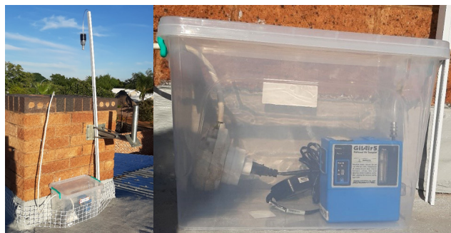
Figure 2: Sampling setup on the roof of a residential building showing the GilAir5 pump, cyclone and the filter cassette.
