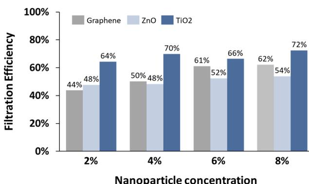
Figure 7: Increase in nanoparticle concentration improves filtration efficiency.  $TiO_2$  has the overall highest filtration efficiency, while Graphene demonstrates the strongest correlation in filtration efficiency and concentration.
