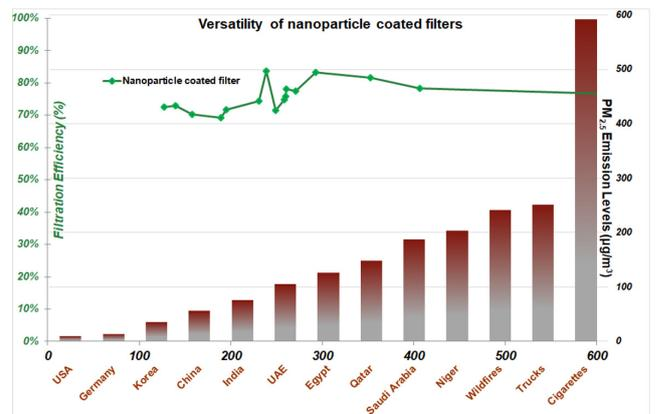
**Figure 14:** Versatility of nanoparticle coated filters in different global pollution levels. The bar-chart indicates the different PM<sub>2.5</sub> levels in different countries and from different sources. The line graph indicates the filtration efficiency relative to the inlet PM<sub>2.5</sub> levels, indicating relatively consistent filtration efficiency over a wide range of PM<sub>2.5</sub> levels (100–600 µg/m<sup>3</sup>).
