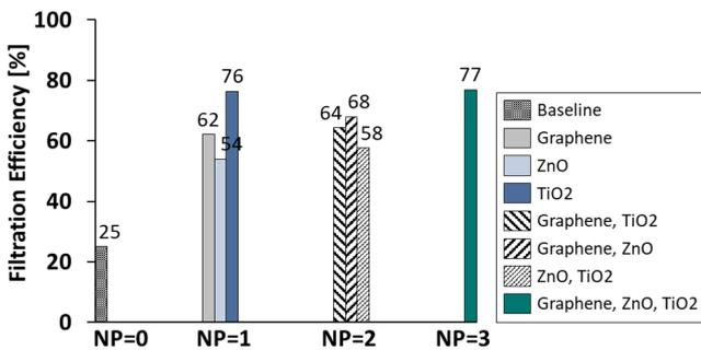
**Figure 12:** Filtration efficiency of nanoparticle coated filters improved significantly relative to a baseline uncoated filter. The Graphene, ZnO, TiO<sub>2</sub> combination is 3 times more effective than a baseline uncoated filter.
