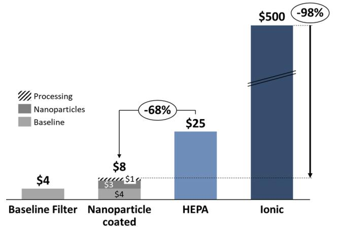
**Figure 13:** Adding the costs of the nanoparticles and processing costs to a baseline filter, the coated filters are significantly less expensive than HEPA or ionic filtration systems.
