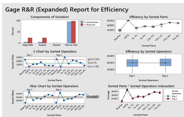
Figure 6: The Gage Repeatability and Reproducibility analysis of the experimental set-up indicating acceptable levels (5% of total variation) of measurement uncertainty.
