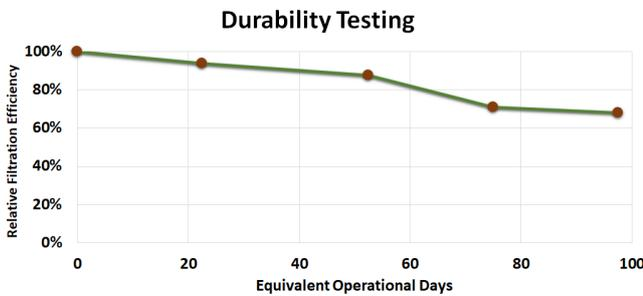
**Figure 11:** Relative filtration efficiency maintained up to 90% of the initial efficiency during accelerated durability testing over 50 equivalent days.
