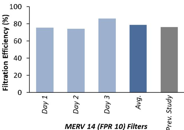
Figure 5: Commercially available MERV14 filters’ filtration efficiency was maintained over different days of testing and was found to be consistent to a previous study, thus confirming the validity of the experimental set-up.
