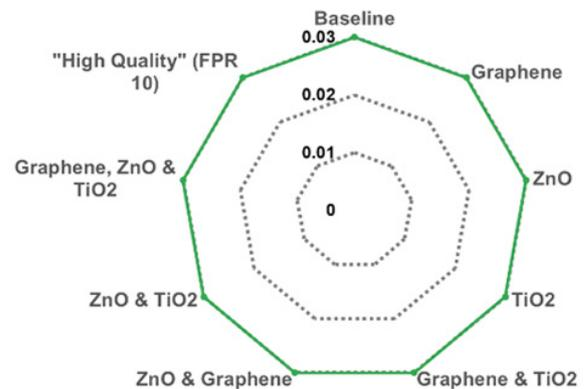
Figure 10: Nanoparticle coated filters have no measurable impact on the pressure drop.
