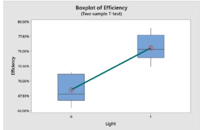
Figure 9: A 2-sample t-test demonstrating impact of light on filtration efficiency of TiO<sub>2</sub>.
