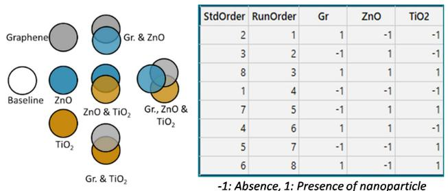
Figure 4: Design of Experiments set-up using full-factorial design for ANOVA analysis. The table indicates the run order used to randomize the experimentation to avoid bias. The figure on the right illustrates the different combinations of the nanomaterials used for the experiment.
