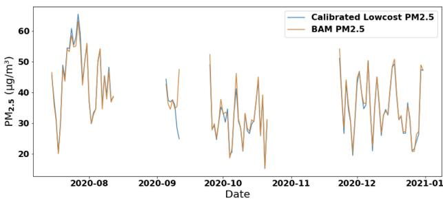
Figure 2: PM<sub>2.5</sub> comparisons for AirQo device AQ88 vs BAM collocated at Makerere University
