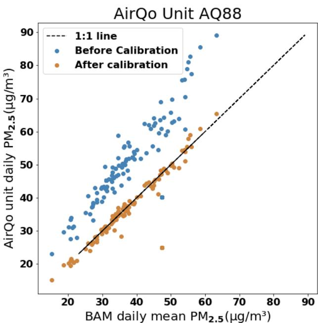
Figure 3: A scatter plot showing the relationship between BAM and AirQo unit PM<sub>2.5</sub> before and after calibration.
