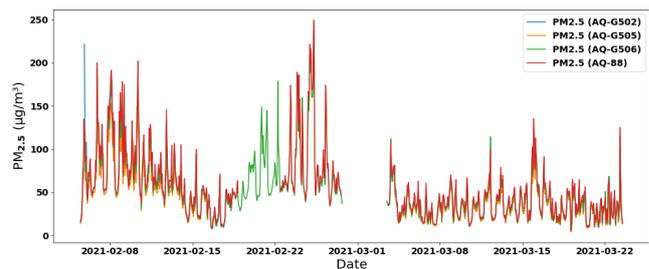
Figure 4: Comparison between hourly PM<sub>2.5</sub> values between AirQo devices collocated at Makerere University
